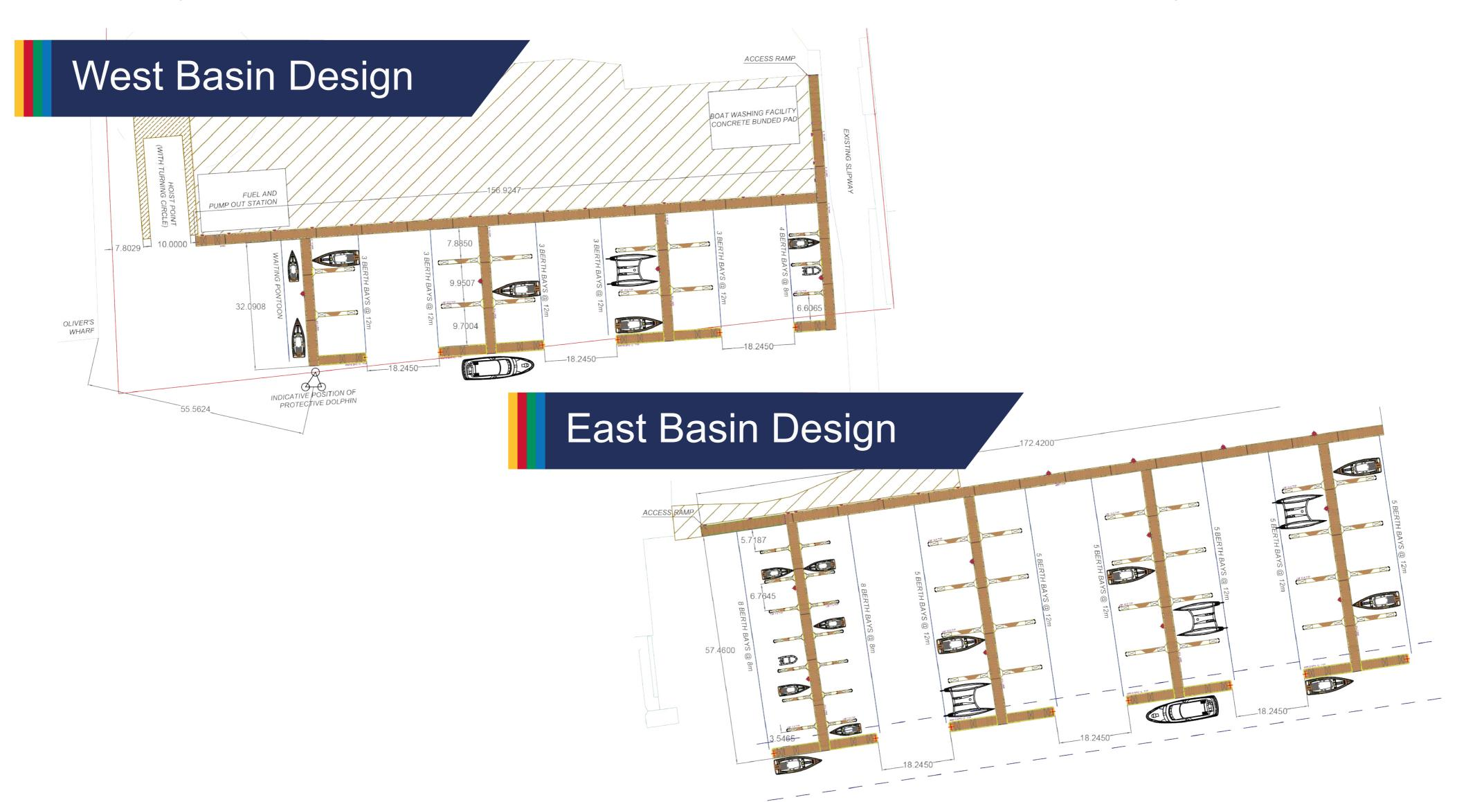
As part of the development, Colne Marine will see the addition of 25 new moorings and the reconfiguration of 90 existing moorings with approximately 275m of new piling in the west basin and 105m in the east basin will be constructed. This new piling will replace the rotted and decrepit telephone poles, to increase site security and longevity.
